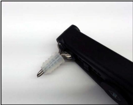
FIGURE 11 - PROTECTIVE SHROUD PLACED ON TOOL
