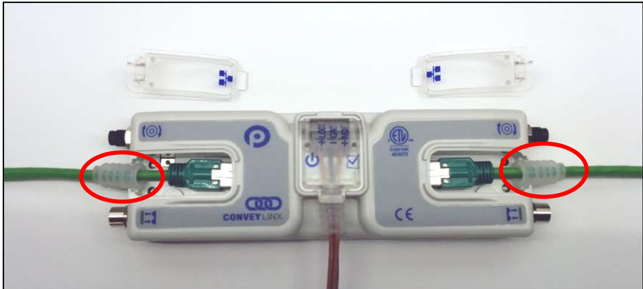
FIGURE 8 – CONVEYLINX-AI2 WITH LEFT & RIGHT ETHERNET CABLES (COVERS REMOVED)
