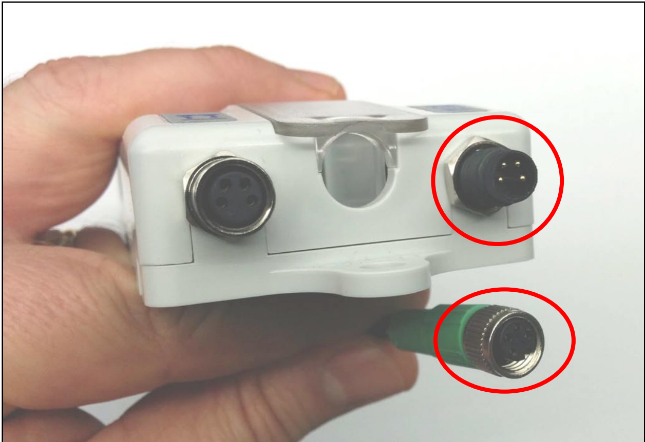
FIGURE 3 - M8 MALE RECEPTACLE AND SENERGY-AI2 FEMALE CONNECTOR
