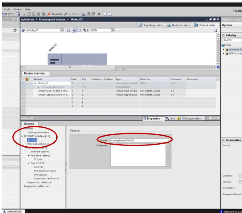
Select *Ethernet Addresses* and select you PLC's subnet and enter the I.P. address of the module you are adding. In this case it is "192.168.200.21".
