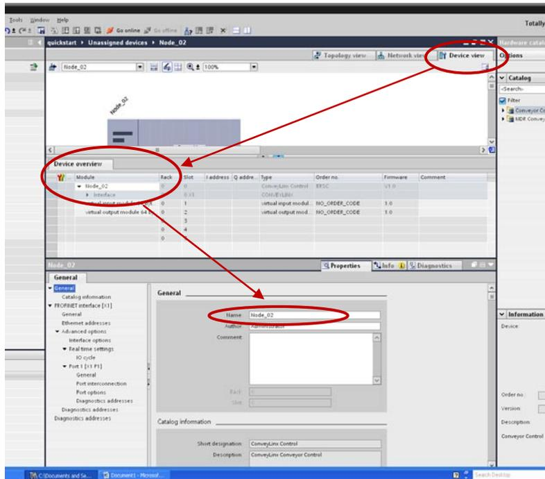
Select "General" under the "Profinet Interface" and enter in the exact Profinet Name syntax for the specific module. In this case we enter "conveylinxplc-200-21"
