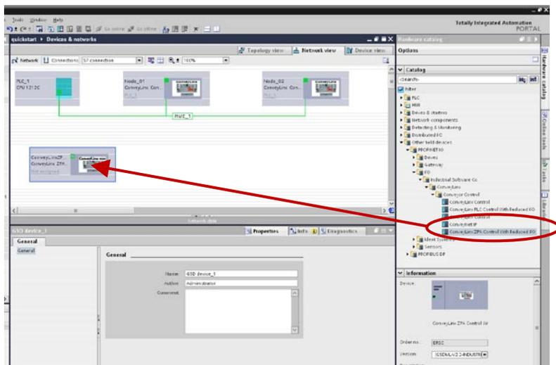
Similarly as previous modules, enter the *Profinet Name* for the module in the “General” area of the “Profinet Addresses” selection. In this case the Profinet Name is “conveylinxzpa-200-22”
