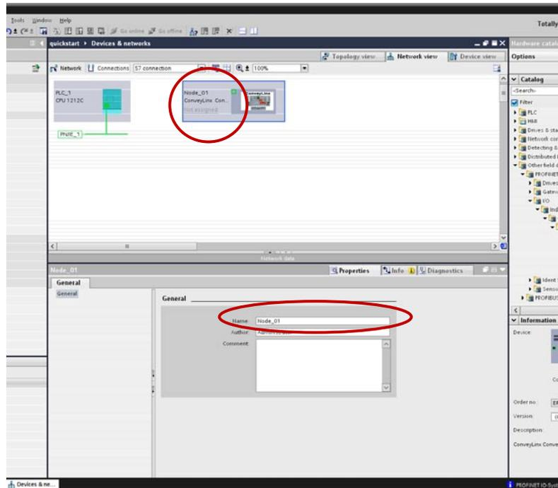
Double click the module icon to open the Profinet Interface settings and select "General" and enter in the exact Profinet Name syntax for the specific module. In this case we enter "conveylinxpa-200-20"
