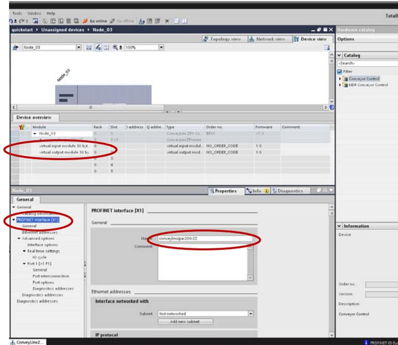
**ADD REDUCED PLC CONTROLLED MODE MODULE**
