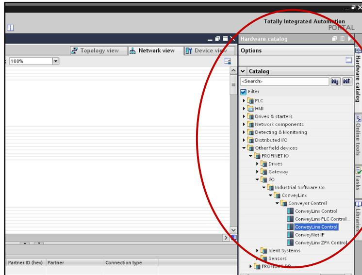
The Mode of operation of a given ConveyLinX module will determine which of the devices do drag and drop from the Hardware Catalog window into your project. Also, once the module has been dragged and dropped into your project, there are other parameters to enter to tell the PLC what Mode of operation you wish to use for the given module.
