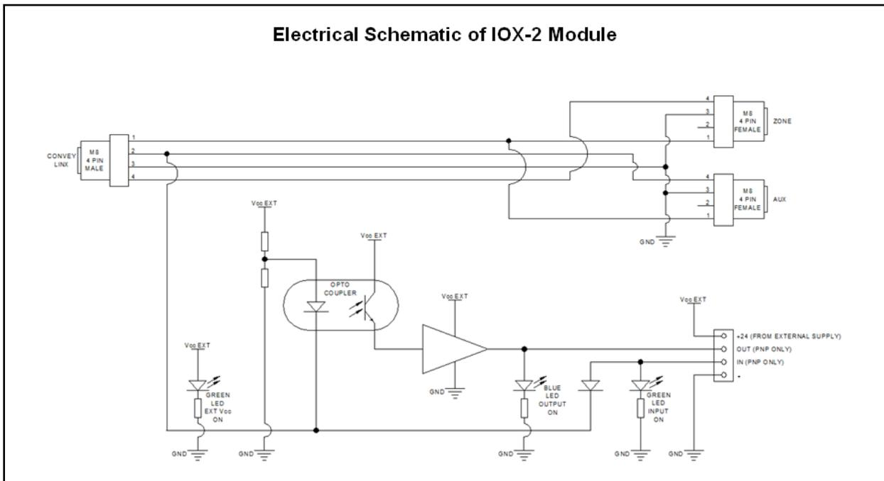
FIGURE 29 - ELECTRICAL SCHEMATIC OF IOX-2 MODULE
