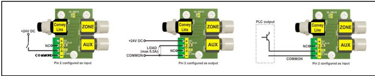
FIGURE 28 - TYPICAL CONNECTION WIRING DIAGRAMS
