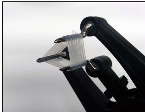
FIGURE 11 - SHROUD STRETCHED WITH TOOL
