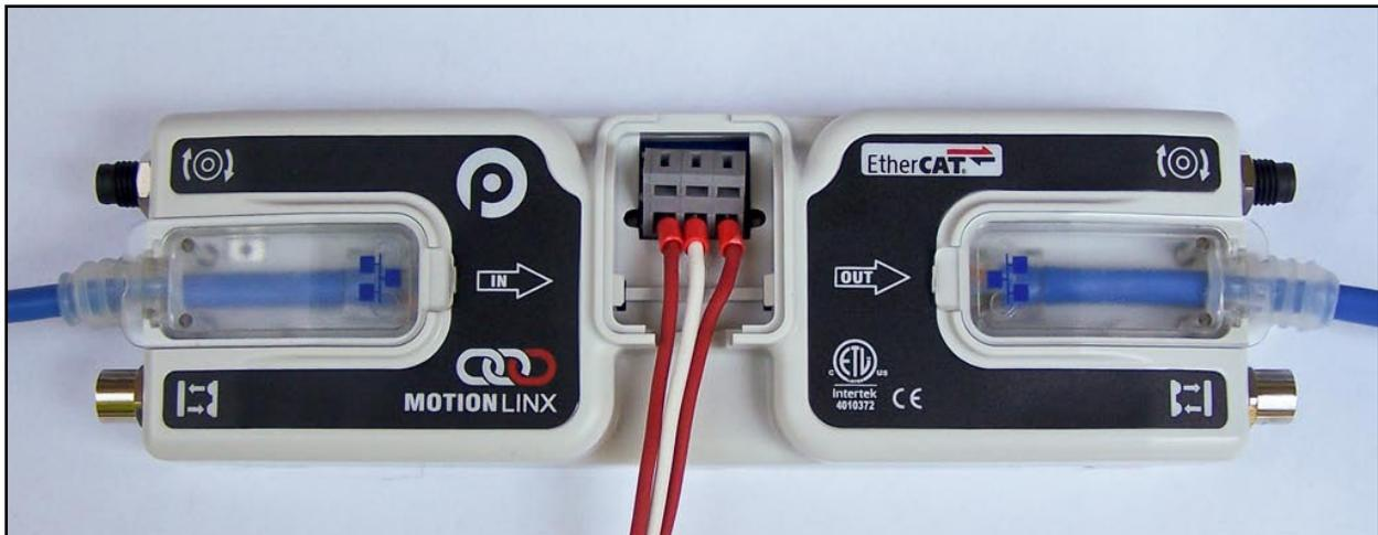
FIGURE 7 - ETHERNET CABLES CONNECTED WITH COVERS ATTACHED
