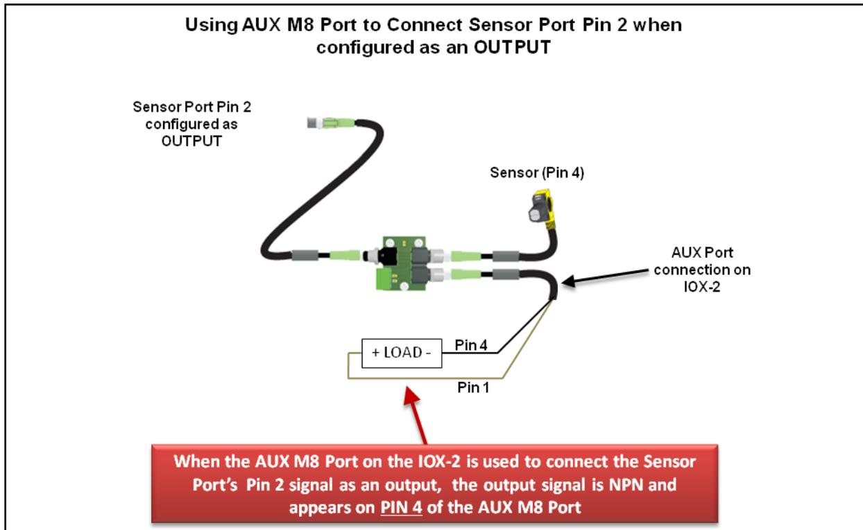
FIGURE 26 - AUX M8 PORT USED WHEN SENSOR PORT PIN2 IS CONFIGURED AS OUTPUT
