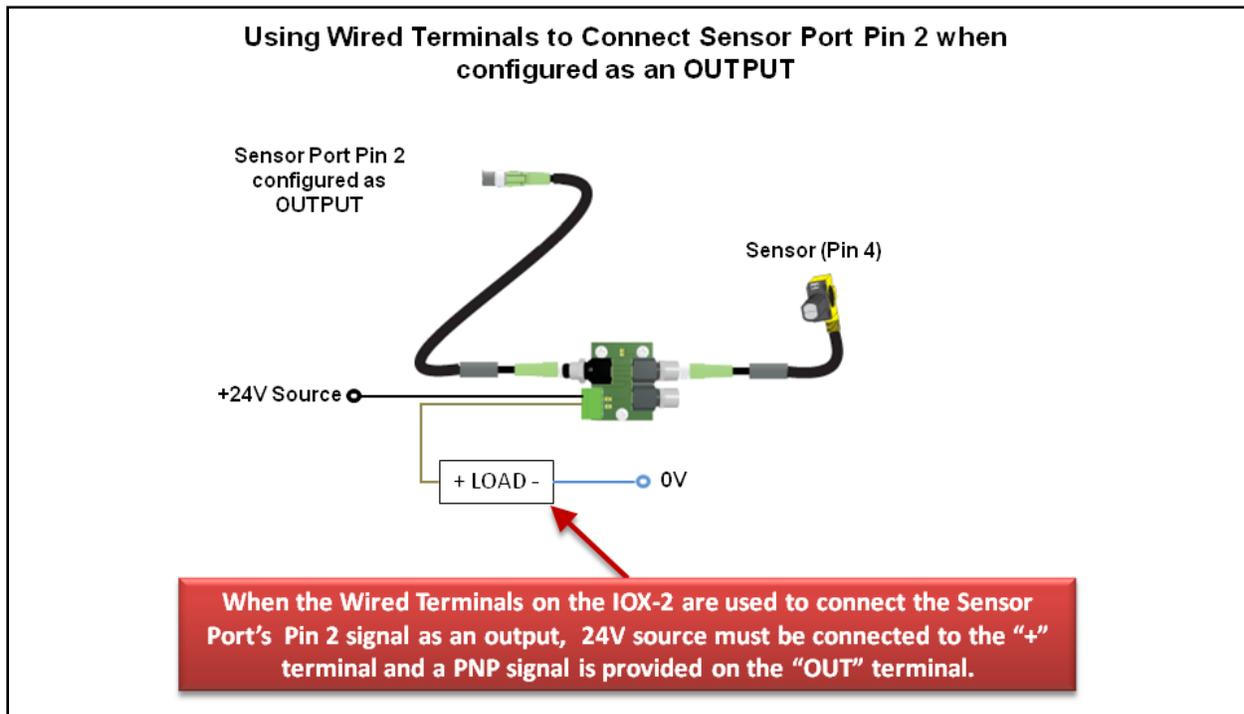
FIGURE 27 - USING WIRED TERMINALS FOR SENSOR PORT PIN 2 CONFIGURED AS AN OUTPUT
