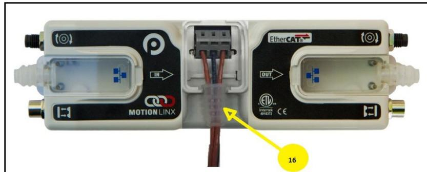
Once wiring has been completed the power wiring compartment is then sealed by snapping into place the Power Compartment Cover (Item 12).
