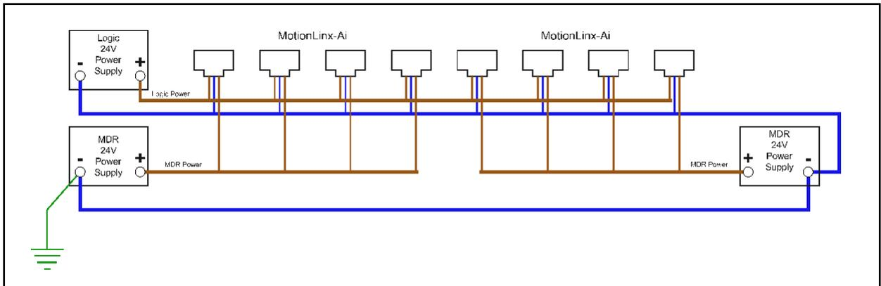
FIGURE 17 - DUAL POWER SUPPLY CONNECTION WITH DC COMMONS TIED TOGETHER AND TO GROUND
