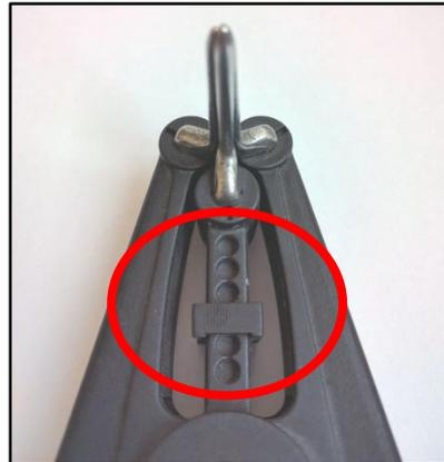
FIGURE 9 - TOOL SHOWN WITH PROPER SET STOP POSITION
