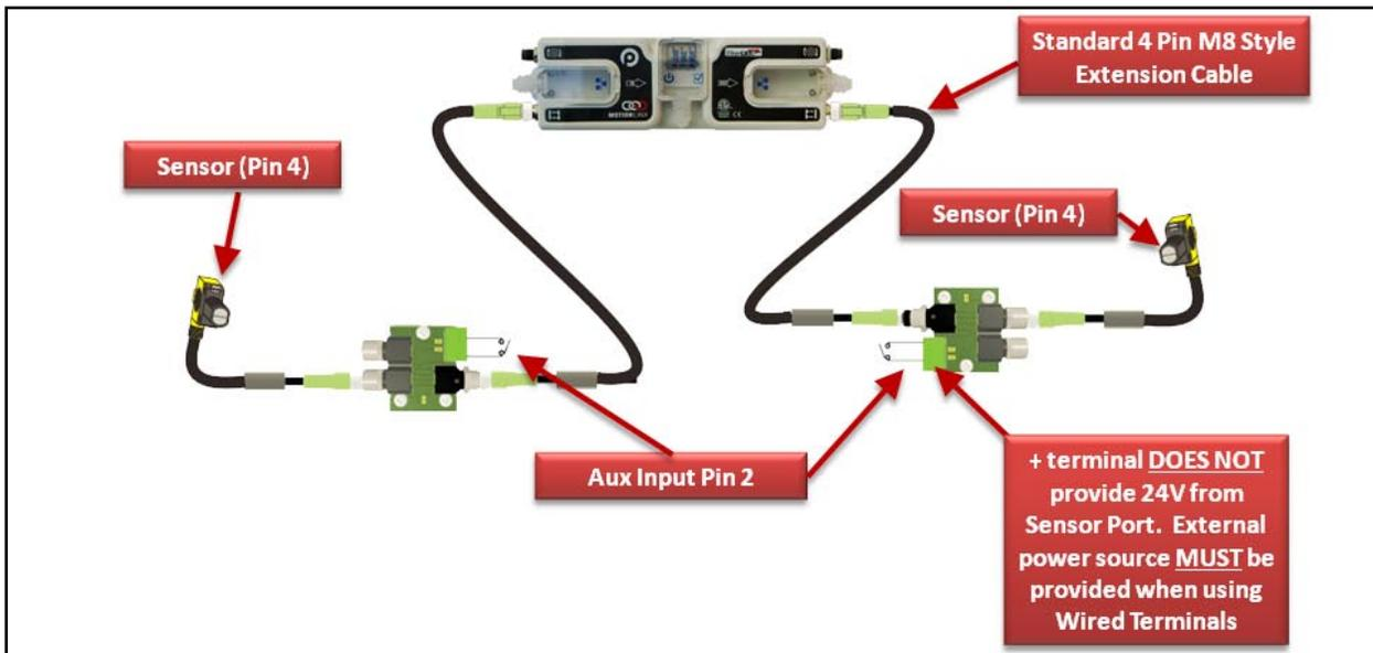
FIGURE 25 – 2 M8 SENSORS AND 2 SWITCH CONTACTS WIRED TO TERMINALS
