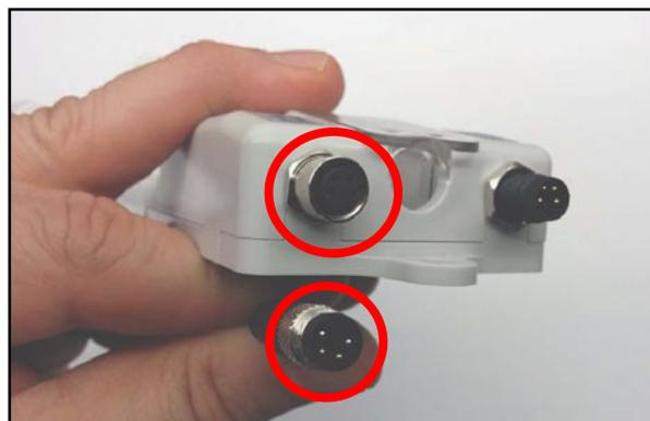
FIGURE 5 – MOTIONLINX-AI FEMALE SENSOR PORT AND MATING SENSOR'S MALE CONNECTOR
