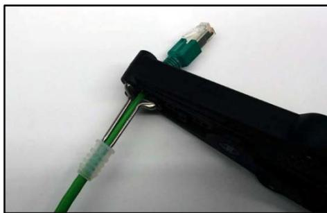
FIGURE 13 - SHROUD REMOVED FROM TOOL PINS
