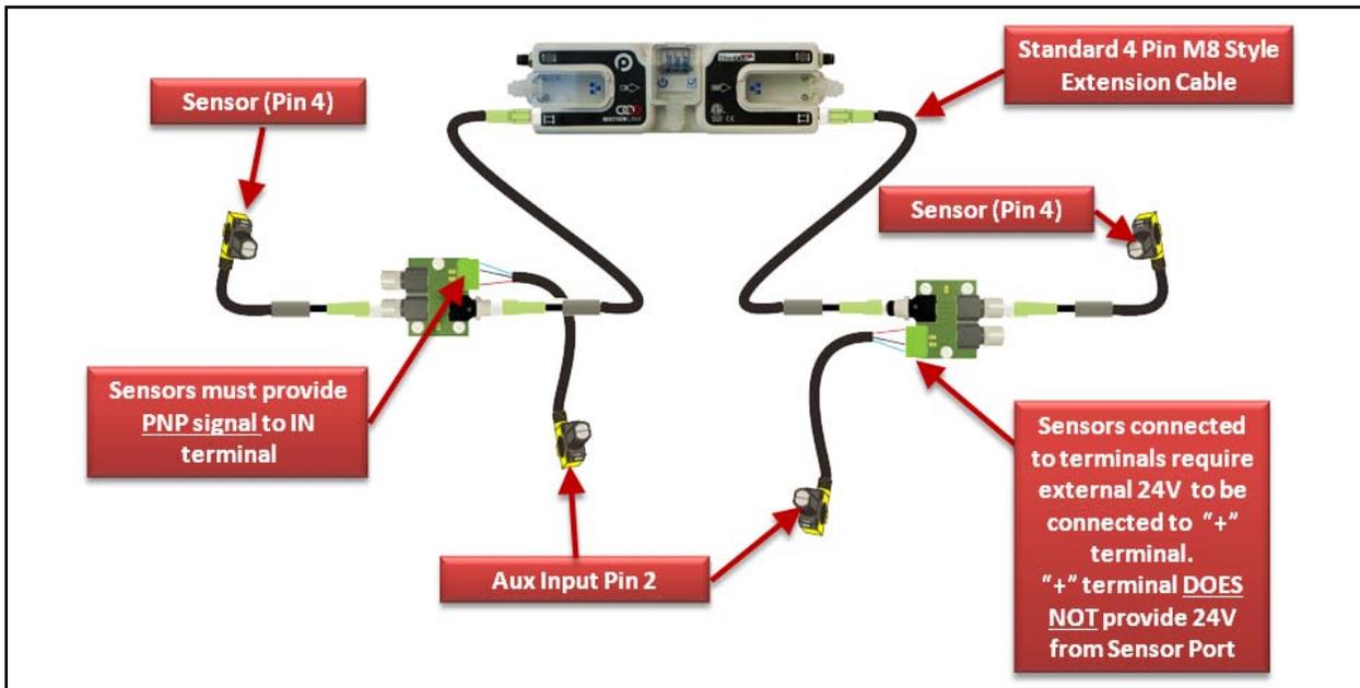
FIGURE 24 – 2 M8 SENSORS AND 2 SENSORS WIRED TO TERMINALS
