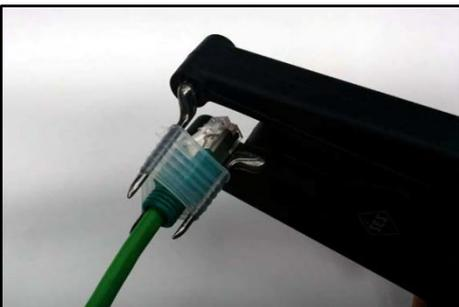
FIGURE 12 - INSERTING RJ-45 END THROUGH SHROUD
