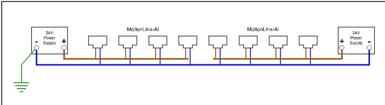
FIGURE 16 – SINGLE POWER SUPPLY CONNECTION WITH DC COMMONS TIED TOGETHER AND TO GROUND
