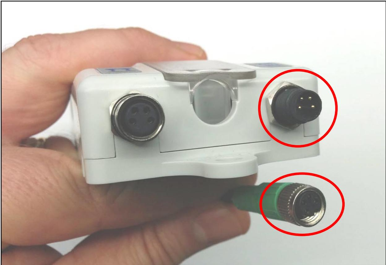
FIGURE 3 - M8 MALE RECEPTACLE AND SENERGY-AI FEMALE CONNECTOR
