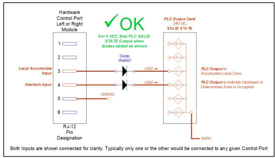
FIGURE 34 - DIODE CONNECTION POLARITY FOR SOLID STATE SINKING OUTPUT MODULE
