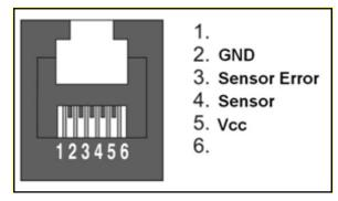
FIGURE 5-CONVEYLINX SENSOR PORT DIAGRAM
