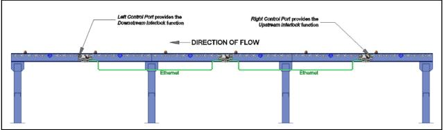
FIGURE 20 - CONTROL PORT ASSIGNMENT EXAMPLE BASED UPON OPPOSITE FLOW DIRECTION
