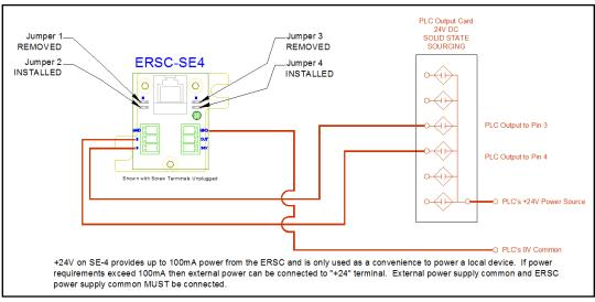
FIGURE 39 - TYPICAL PLC SOURCING OUTPUT CONNECTION TO ERSC INPUTS
