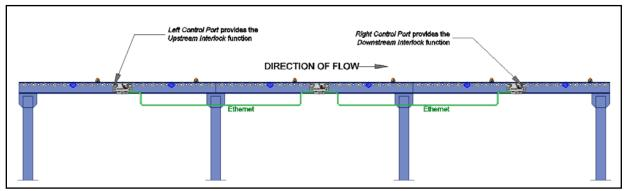
FIGURE 19 - CONTROL PORT ASSIGNMENT BASED UPON FLOW EXAMPLE
