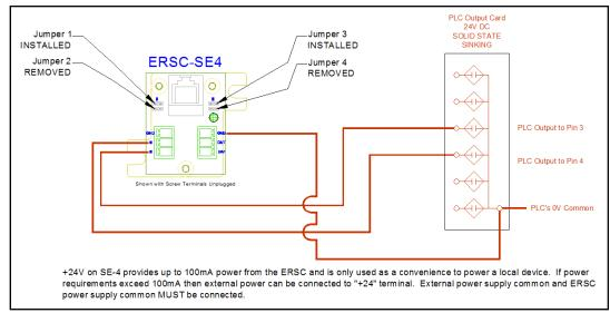
FIGURE 40 - TYPICAL PLC SINKING OUTPUT CONNECTION TO ERSC INPUTS
