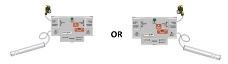
In this example, a single MDR and photo-sensor is connected to either the Left or Right group of ports. The module controls the MDR as a single independent logical conveyor zone.
