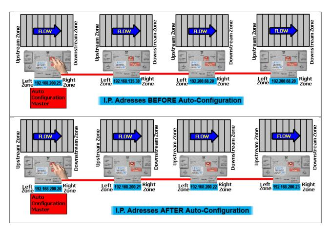
The Auto-Configuration Procedure will assign Nodes up to and including Node 240. Therefore each Subnet is limited to 220 ERSC Nodes.
