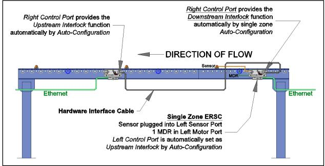
FIGURE 23 - SINGLE ZONE HARDWARE INTERFACE EXAMPLE
