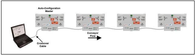
FIGURE 41 - INITIAL PC CONNECTION TO CONVEYLINX SUBNET
