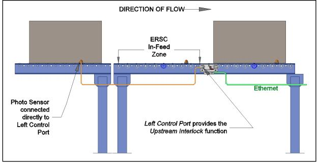
FIGURE 25-SENSOR IN UPSTREAM INTERLOCK CONTROL PORT EXAMPLE
