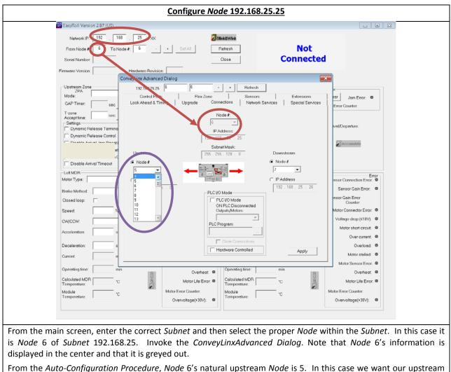
From the Auto-Configuration Procedure, Node 6's natural upstream Node is 5. In this case we want our upstream zone to be fed from Node 4 instead of Node 5 because Node 5 will be our Slave zone. For the Upstream zone, select Node 4 from the pull down box and click apply.
