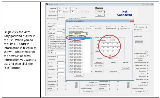
After clicking the "Set" button, you can click the "Discovering" button again and *EasyRoll* will refresh the list of modules at the left. You can verify that the module has the new I.P. address settings.
