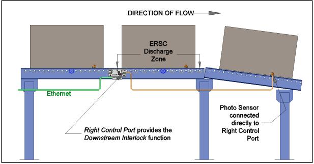
FIGURE 24-SENSOR IN DOWNSTREAM INTERLOCK CONTROL PORT EXAMPLE
