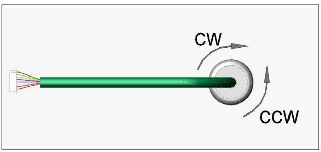
FIGURE 11 - MOTOR ROTATION DIRECTION CONVENTION
