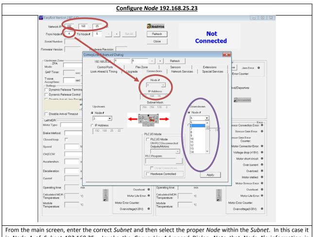
is Node 4 of Subnet 192.168.25. Invoke the ConveyLinxAdvanced Dialog. Note that Node 4's information is displayed in the center and that it is greyed out.
