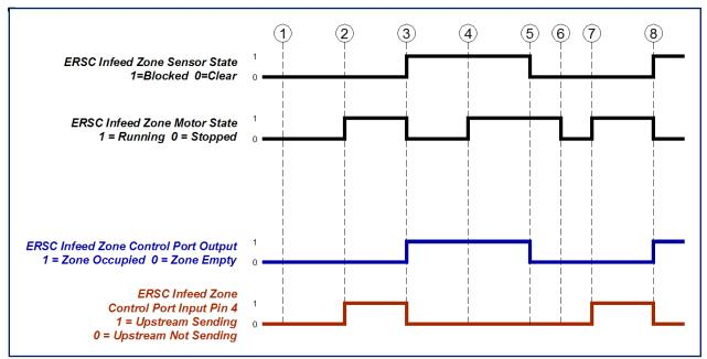
FIGURE 27 - TYPICAL UPSTREAM INTERLOCK TIMING EXAMPLE
