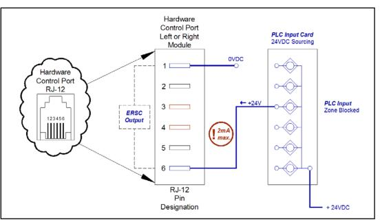
FIGURE 31 - SOURCING PLC INPUT FROM ERSC CONTROL PORT OUTPUT
