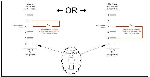
FIGURE 18- ACCUMULATE CONTROL CONNECTION EXAMPLES
