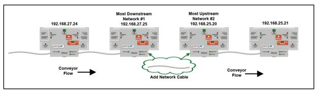
FIGURE 50 - SUBNET BOUNDARY EXAMPLE WITH CABLE
