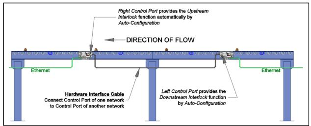
FIGURE 21 - TYPICAL HARDWARE INTERFACE CABLE EXAMPLE
