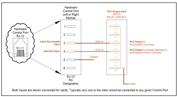
FIGURE 33 - SINKING PLC RELAY CONTACT OUTPUT TO SINKING ERSC CONTROL PORT INPUT
