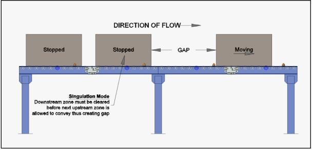
FIGURE 16 - SINGULATION RELEASE EXAMPLE
