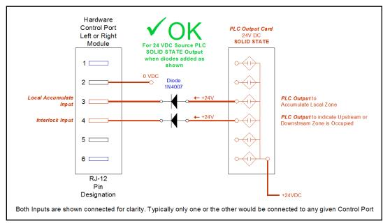
FIGURE 35 - DIODE CONNECTION POLARITY FOR SOLID STATE SOURCING OUTPUT MODULE
