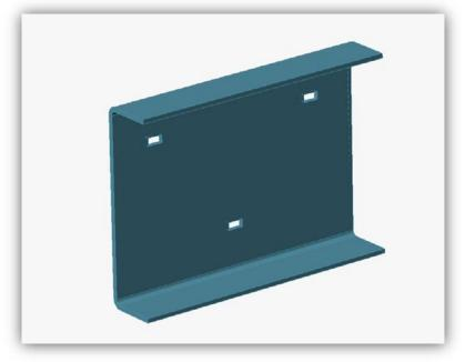
FIGURE 52 - PERFORATION PATTERN FOR CONVEYOR SIDE FRAME
