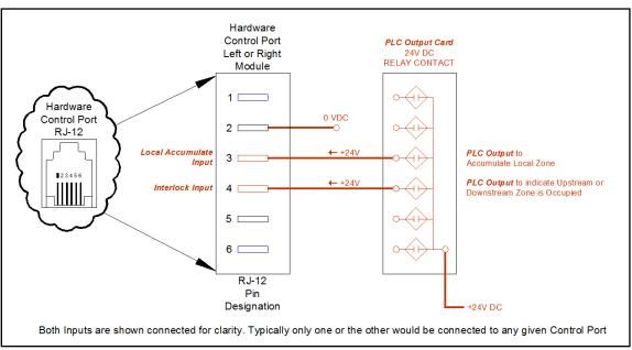
FIGURE 32 - SOURCING PLC OUTPUT TO SINKING ERSC CONTROL PORT INPUT
