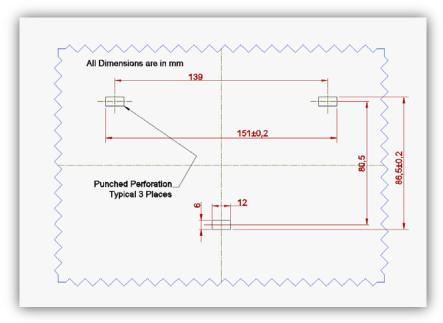
FIGURE 51 - CONVEYOR SIDE FRAME ELEVATION VIEW OF PERFORATION
