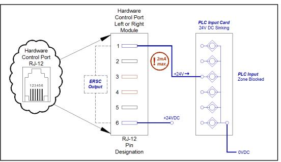
FIGURE 30-SINKING PLC INPUT FROM ERSC CONTROL PORT OUTPUT
